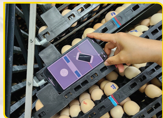
Measuring turning angles using an app such as Angle Meter Pro.
